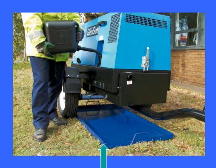
Spillage could have been avoided by using a Drip tray.
