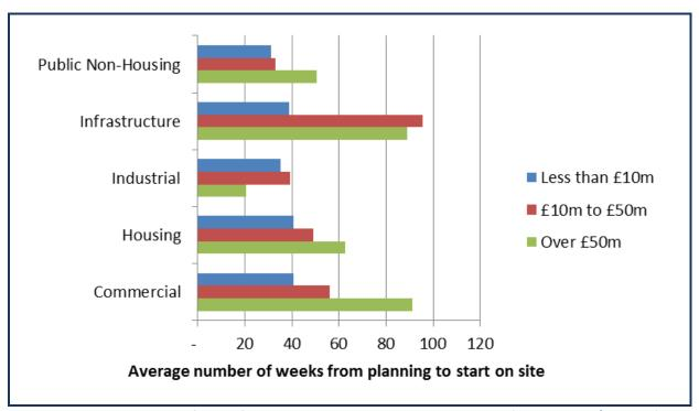
Figure 10: Average number of weeks from planning to work on site, UK 2010-2013 (Source: UKCG/Glenigan)
